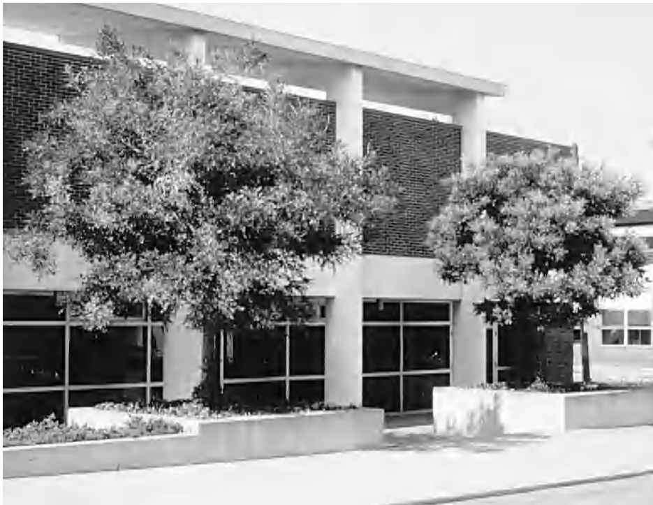
Fig. 24. Raised planters can be used to provide more soil volume, avoid road salt and other runoff, and provide shady seats. The bottoms of raised planters should be kept open.
