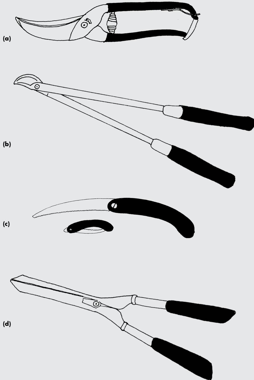
**Figure 2.** Examples of the most common tools required for pruning small ornamental trees and shrubs, including hand pruners (a), lopping shears (b), pruning saws (c), and hedge shears (d).
