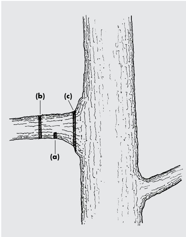
**Figure 10.** Removing larger branches safely and avoiding greater injury to the tree requires three cuts. The first cut (a) is made from the bottom of the limb about 10 to 12 inches from the trunk. The second cut (b) is from the top, 3 to 4 inches out from the first cut. The third cut is down and out from the branch collar, thus removing the remaining stub and ensuring that the pruning wound closes properly.
